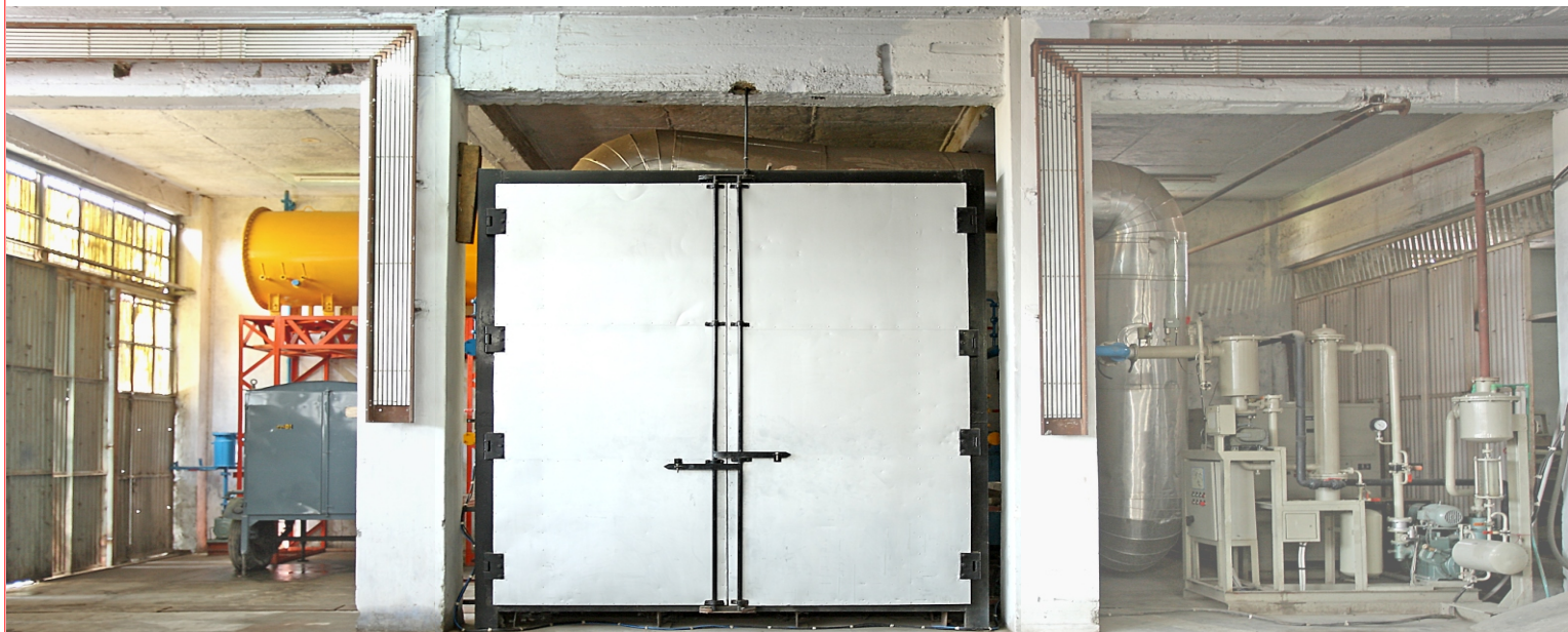
High Vacuum Controlled Heat Arrangement Chamber with Built in Duty Vacuumed Oil Filling in Instrument Transformer
